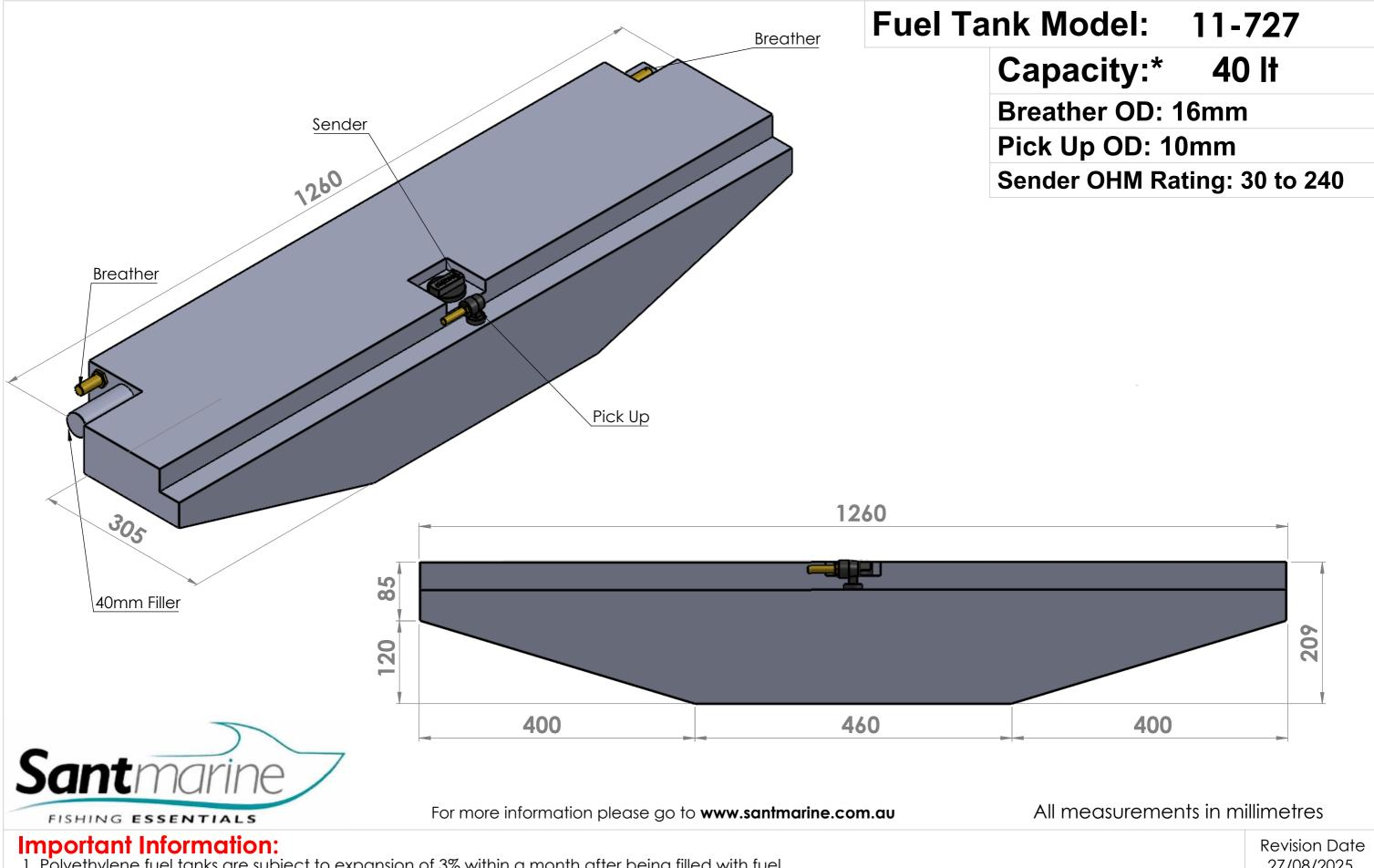
Polyethylene fuel tanks are subject to expansion of 3% within a month after being filled with fuel.
